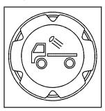
This button is located on the driver side of the instrument panel near the exterior lamp control.
